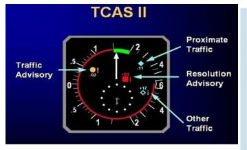
How does TCAS work? It gets signals from other aircraft, equipped with RBS or Mode-S transponders, shows these aircraft to the pilots on a special indicator (usually on a Navigational Display or EHSI — Electronic Horizontal Situation Indicator), monitors the airspace around an aircraft, analyses movements of other traffic and if necessary, gives commands either to climb or to descend in order to avoid near-miss or collision with other aircraft
