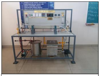
CONCENTRIC TUBE HEAT EXCHANGER
