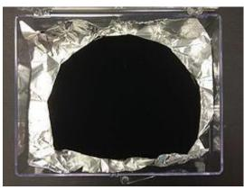
Fig. 1: Aluminium foil with a portion coated in Vantablack
